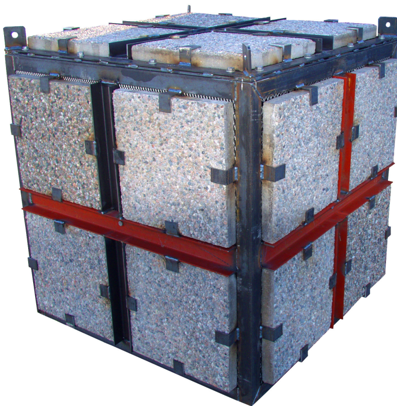
Figure 14 1 m cubic object used for verification of object detection performance.
