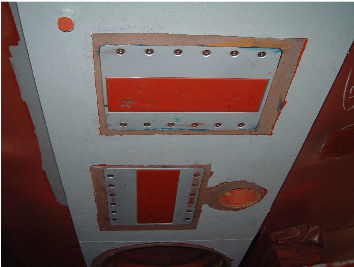
Figure 18 Installation of the 2x2 degrees transducer array on “HMS Endurance”
